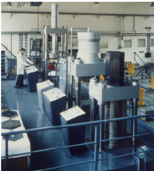
Fig. 5 Pilot Plant for Fabrication of HTR Moulded Block Fuel Elements (upper working level)
