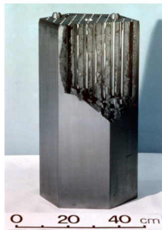
Fig. 5 Molded Block FE with embedded Coated Particles, Heavy Metal = 18kg
